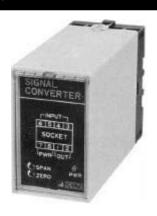
This instrument is a high accurate converter which provides simultaneously power supply and signal conversion to all transmitters such as pressure transmitter, flow transmitter, level transmitter, etc and contains overcurrent and overvoltage protection circuit inside. It is isolated between signal transmitted from transmitter and output signal of converter, not necessary to use extra isolator when loop constructing.
