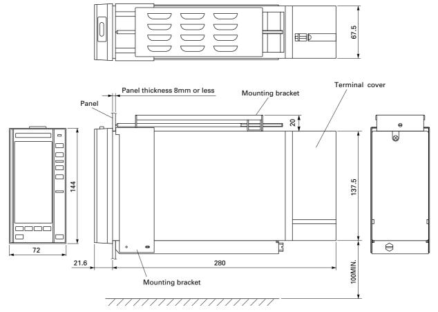
Note) The distance between other instruments and low end of PDF shall be more than 100mm.
