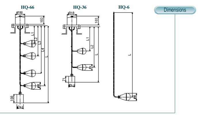
Let the WEIGHT loosen by inserting from the upper part of tank. Insert FLOAT with GUIDE WIRE
